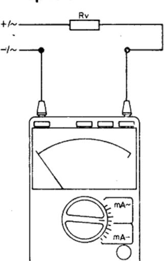
Put measuring range switch (6) into the position 5000 mA— or 5000 mA~.
