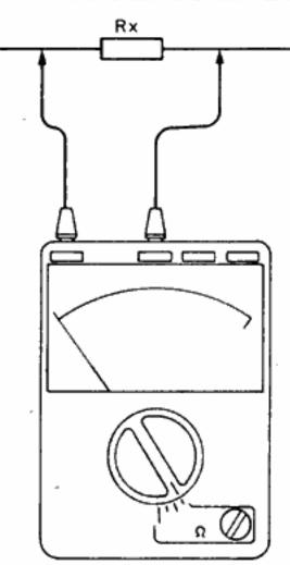
Resistance is measured with direct voltage from the 1.5 V miniature cell used. The measuring range table in Section 3 shows the maximum measuring currents with full deflection and with a battery voltage of 1.5 V.
